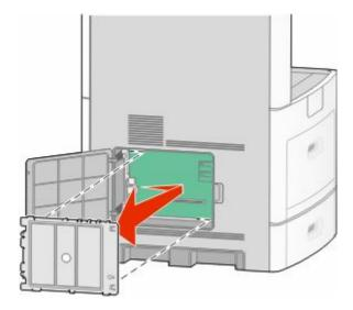
**4** Use the illustration below to locate the appropriate connector.
