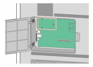
Note: If an optional ISP is currently installed, then the printer hard disk must be installed onto the ISP.
