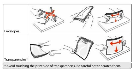
Load the paper or specialty media. Slide the stack gently into the multipurpose feeder until it comes to a stop.
