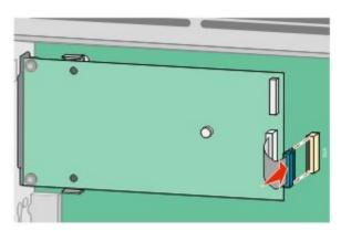
**12** If a printer hard disk was previously installed, then attach the printer hard disk to the ISP. For more information, see "Installing a printer hard disk" on page 37.
