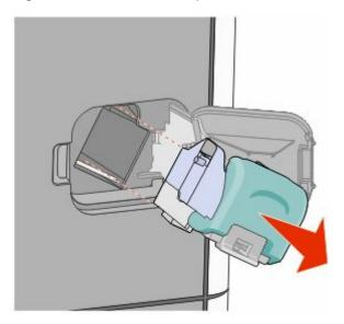
Use the metal tab to lift the staple guard, and then remove any loose staples.
