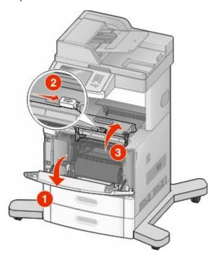
**4** Lift and pull the print cartridge out of the printer.
