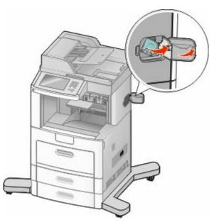
**3** Pull the latch of the staple cartridge holder down, and then pull the holder out of the printer.
