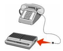
**5** Connect a third telephone cord from the answering machine to the EXT port **1** of the printer.
