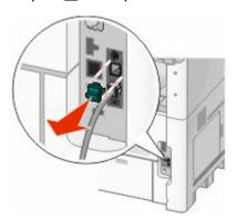
**4** Connect a second telephone cord from the telephone to the computer modem.
