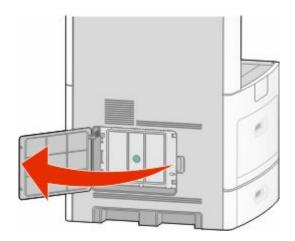
**2** Loosen the screw(s) on the system board cover.
